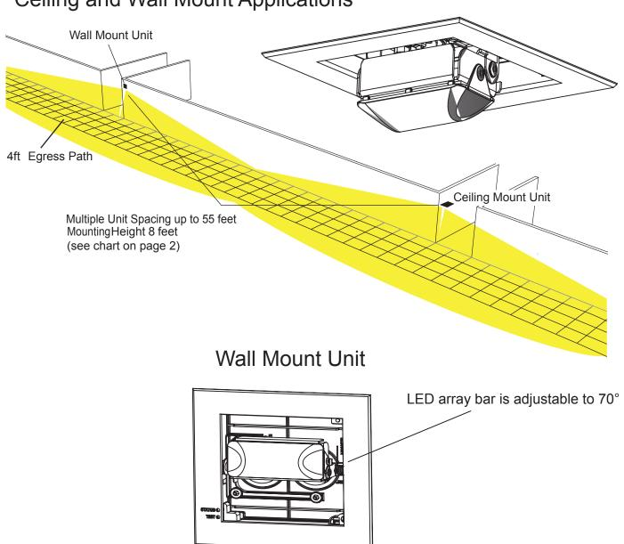
Compliance with the Life Safety Code NFPA 101, Section 7.9.2.1 requires even illumination, over a specified area of 1fc average with a minimum illumination of 0.1fc at any point with a ratio of not more that 40 to 1.
