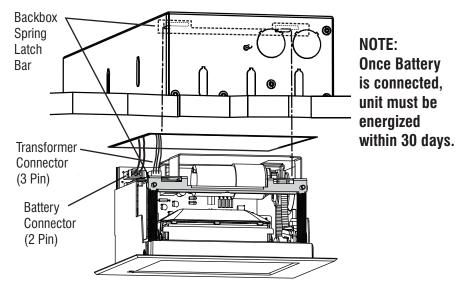
Install lamphead by first locating in place in Backbox opening.
