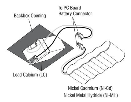
Insert Battery (TERMINALS OR CONNECTORS FACING OUT) through Lamphead opening. Allow Transformer Cable to extend out through Lamphead opening.
