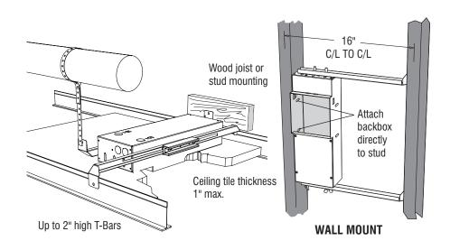
Remove appropriate mounting knockouts on top, bottom or sides of backbox. Attach Bar Hangers to backbox using Bolts and Hanger Clamps supplied.
