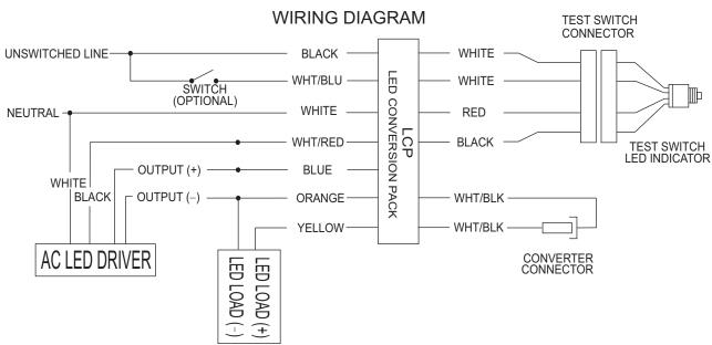
TYPICAL SCHEMATIC ONLY. MAY BE USED WITH OTHER DRIVERS. CONSULT FACTORY FOR OTHER WIRING DIAGRAMS
