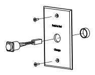
B. For installation of test switch on fixture surface.
