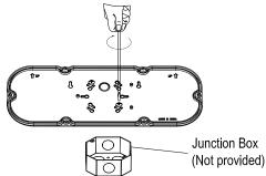
3. Secure emergency lighting fixture backplate to waterproof case back plate, then install the fixture.
