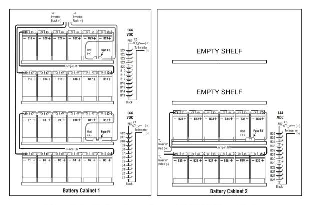
Three String Battery Connection - 144 VDC 3 Phase Systems
