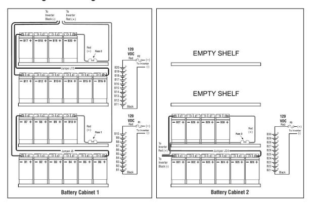
Three String Battery Connection - 120 VDC 3 Phase Systems
